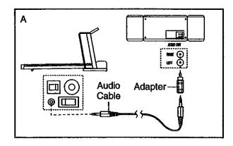
B. Plug one end of the audio cable into the jack on the front of the treadmill near the power cord. Plug the other end of the cable into the LINE OUT jack on your stereo.
